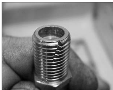
Fig. 2. Thread chaser to clean threads for the petcocks. This is easier to do before the epoxy has set up completely.
